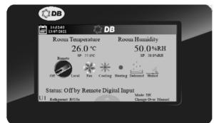
DB-Aire In Row is equipped with a colored touch screen controller for interactive controls and display. The 65k color display provides a high quality images and advanced features for user to conveniently navigate between various screens.
