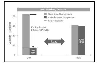
VFD Advantage 2 – Better temperature control compare to conventional fix speed control.
